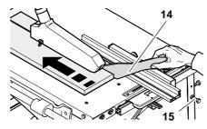
Guide the push stick at an angle of  $20^{\circ}$  ...  $30^{\circ}$  against the saw table's surface.
